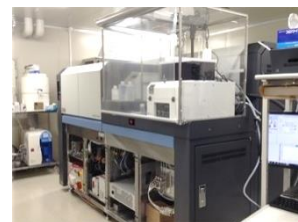
Instrument for measuring mercury isotope ratios with high precision
