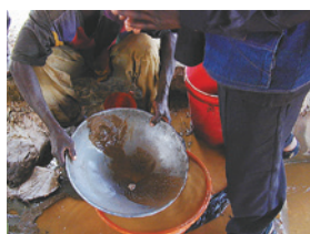
Gold extraction by forming a mercury amalgam in a small scale gold mining
