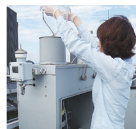
Continuous monitoring of mercury in the rainwater using an automatic wet-only sampler
