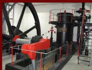
the Idrija Kamšt, the driving wheel of the water-driven pump and the Kley steam pump, Technical department of the Idrija Municipal Museum
